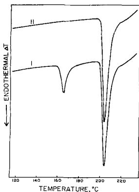
Fig. 2.—Thermograms for forms I and II of sulfathiazole.
